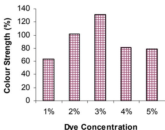
Fig 2. Effect of UV radiation on the colour strength of dye using different concentrations of extracted dye
