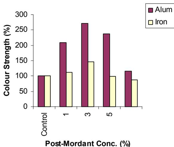
Fig. 4. Effect of post- mordants on the dyeing of cotton using an aqueous extract of UV irradiated turmeric powder
