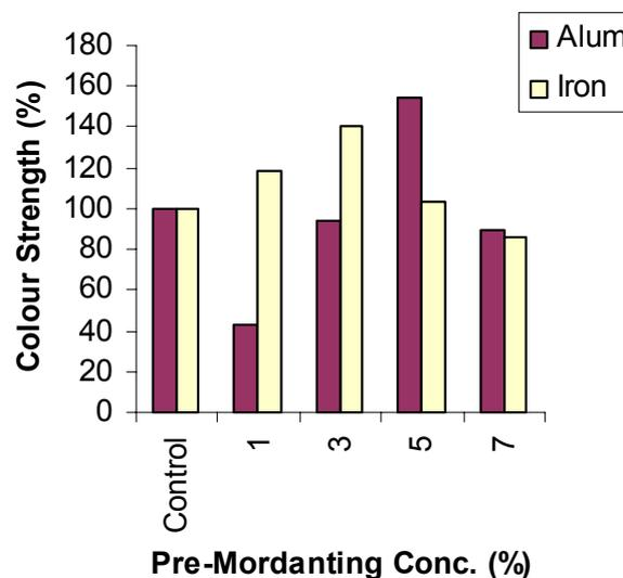
Fig. 3. Effect of pre-mordants on the dyeing of cotton using an aqueous extract of UV irradiated turmeric powder
